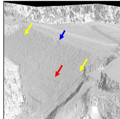
Figure 9: Mesh showing the sliding waves.
