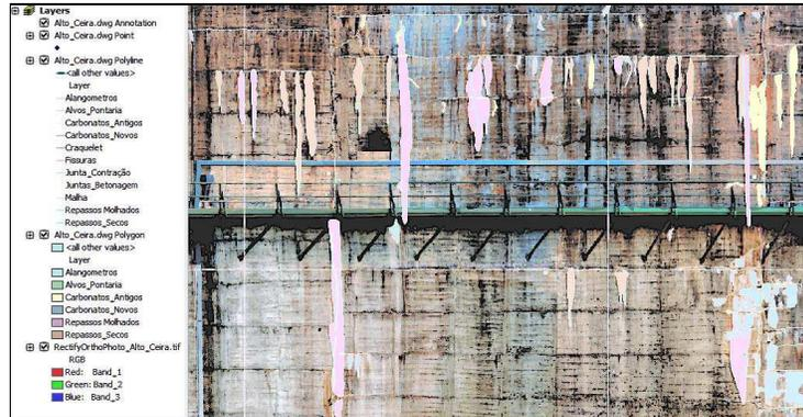
Figure 4 - Association of CAD and DBMS technologies in order to get points, vectors and polygons associated with alphanumeric classifications according to an inspection data catalogue.
