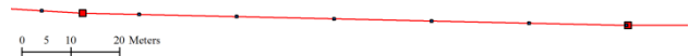
Figure 4. Tunnel axis with the original points (larger squares) and the equally spaced points (small dots).
