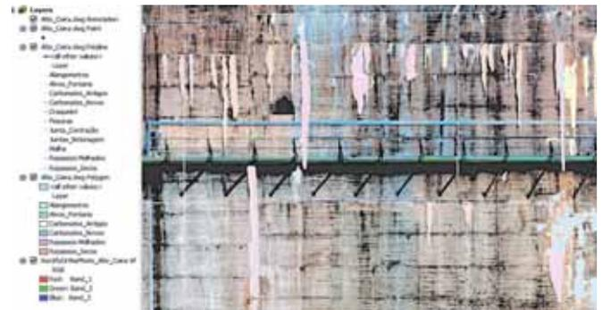
Figure 4: CAD and DBMS technologies were used to get points, vectors and polygons associated with alphanumeric classifications according to an inspection data catalogue.
