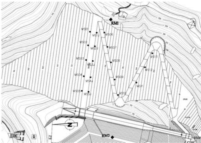
Figure 5. Lapão dam location of reference and object points.
