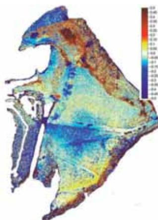
Figure 8: Settlements - 2005 epoch as compared to 2003.
