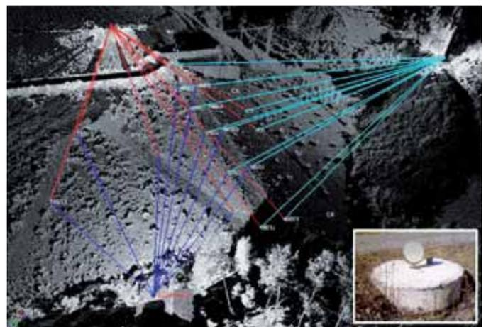
Figure 6: The laser intensity 3D point cloud of the Lapão Dam (2007) showing the three scan positions, retro-reflector targets and vectors between scan positions and surface marks. The smaller image is a retro reflector target.
