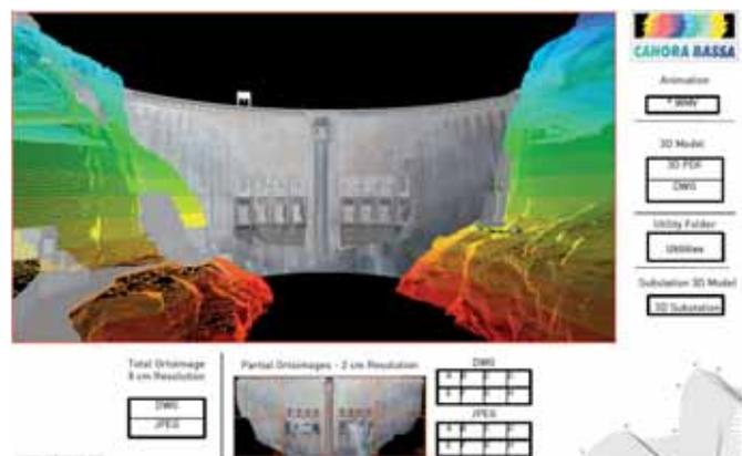
Figure 10: PDF application with embedded 3D CAD model of the Cahora Bassa dam and its near slopes.
