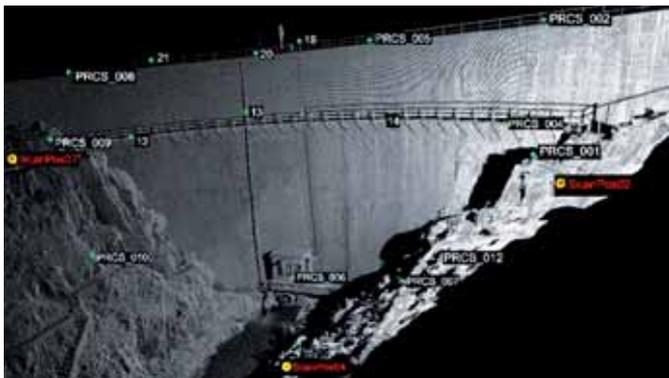
Figure 1: A perspective of the laser intensity 3D model of Alto Ceira dam's downstream face, layout of stations (with red labels) and retro-reflector targets (with white labels).
