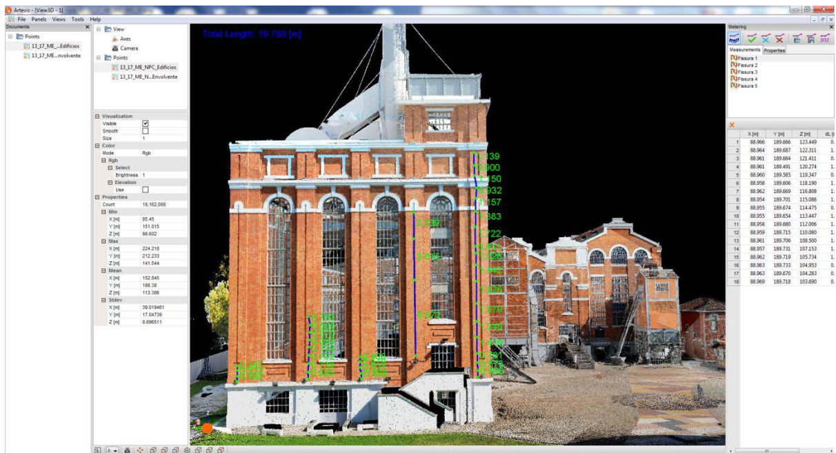
Fig. 4 - 3D Coloured Point Cloud on Artevis, software for the visualization analysis and measurements of point clouds.
